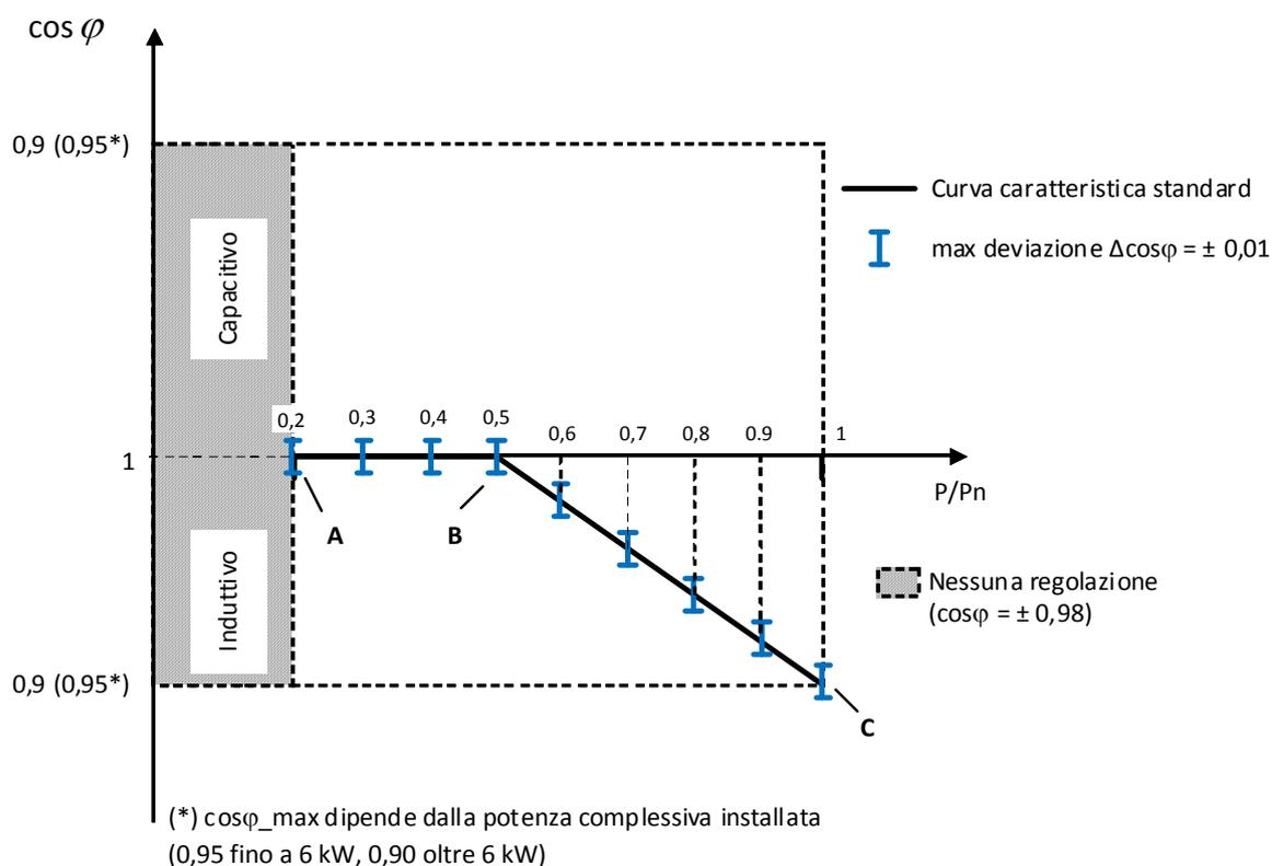
**Figura 27 - Curva caratteristica standard  $\cos\varphi = f(P)$**
